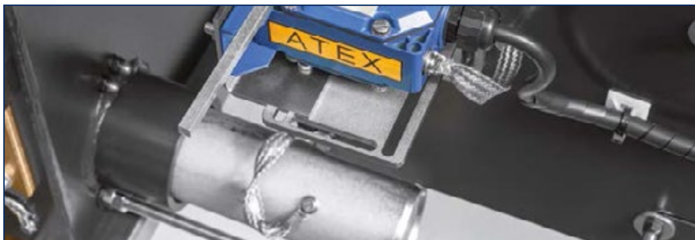
Potential equalisation using earthing strap
