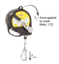
At load weight (Fmax) of 140 kg force applied to the crank (Fk) shall be 6.4 kG.
