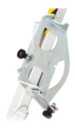
Clamp for mounting retractable type fall arrester CRW 200 on the tripod leg. According to the leg thickness, either clamp AT 173 or AT 174 is used. The clamp is simple to mount and is made of galvanized steel. Above is an example mounting of clamp AT 173 on tripod TM 9 leg.
