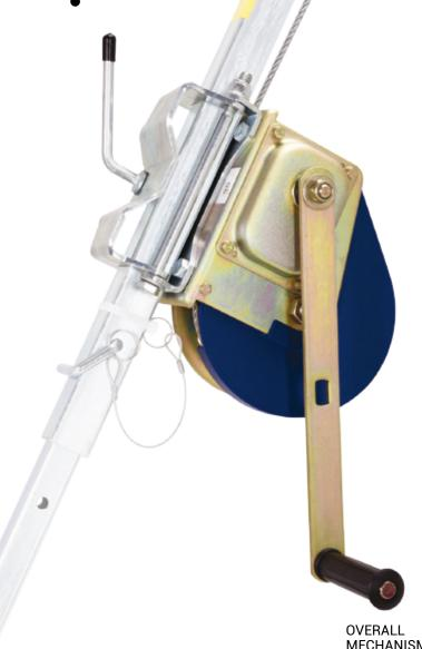
RUP 502-BT is a winch equipped with clamp for mounting on tripod leg. The winch is equipped with six-strand steel cable with natural fibre kern of 25 m in length and 6.3 mm in diameter:
