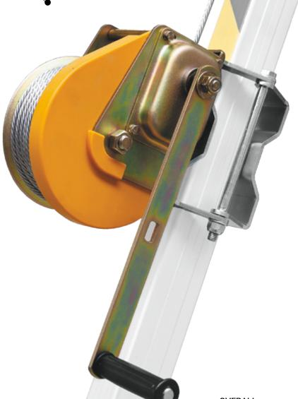
RUP 502-A is a winch equipped with a clamp for mounting on tripod leg. The winch is equipped with six-strand steel cable with natural fibre kern of 20 and 25 m in length and 6.3 mm in diameter;
